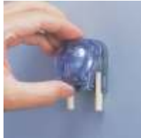
Lift up the pump cover from the bottom side.
