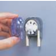
Pull off the pump cover.
