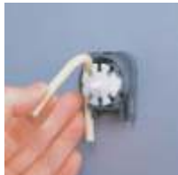
Remove the Squeeze tube. The rotor may come out, but can be pushed back in place.
